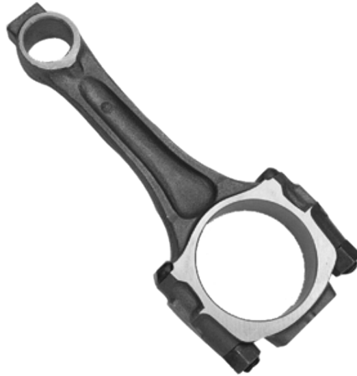
Figure 2.4 (a) Note the two 'ends' of the connecting rod
