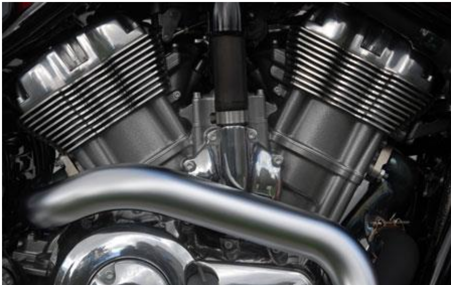
Figure 11.1 Direct cooling system: Motor cycle engines
